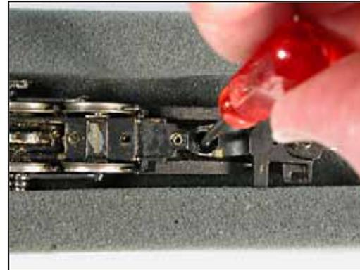
Remove screws connecting to wire lugs
