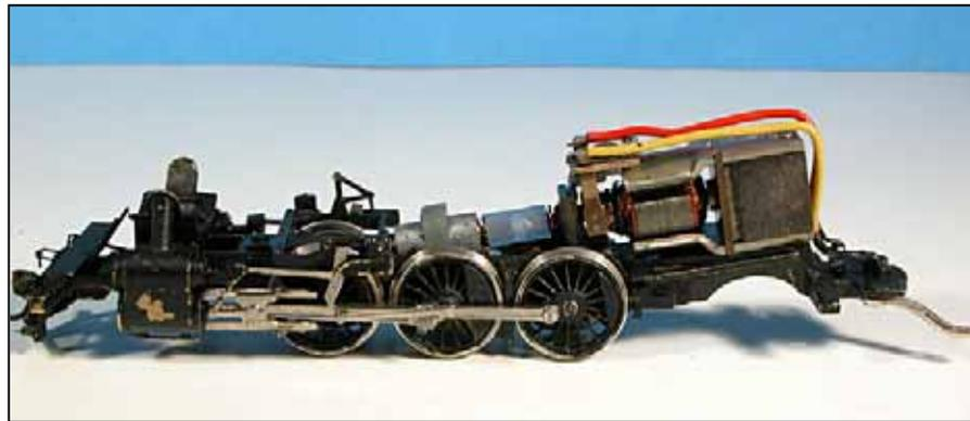
Note new coupling and motor shim.
