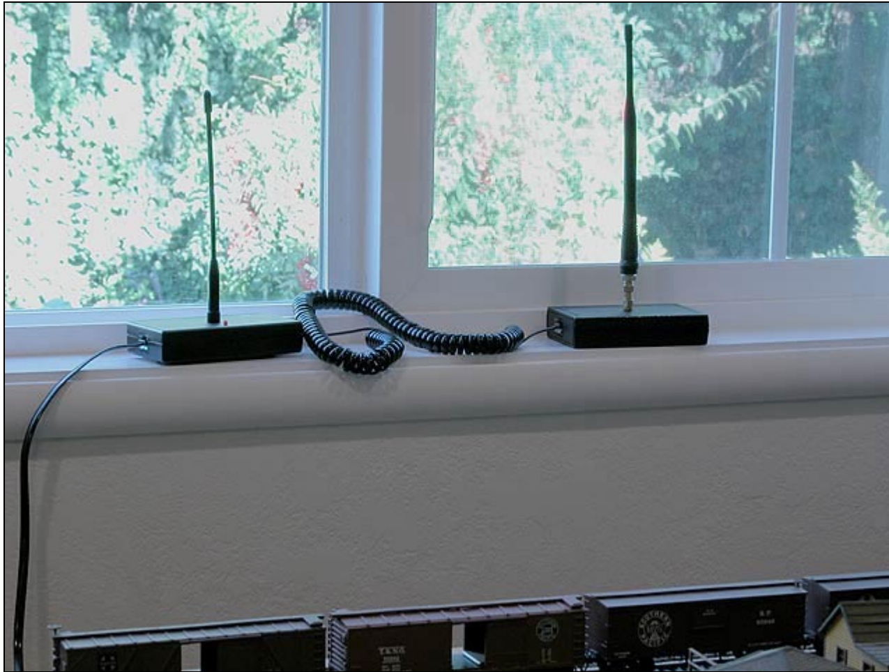
Diversity Receiver in operation on the layout
