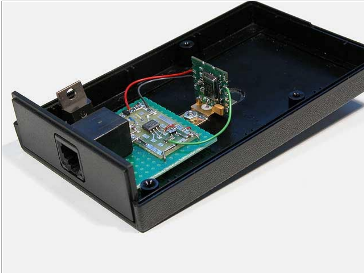
Another view of completed diversity receiver in box
